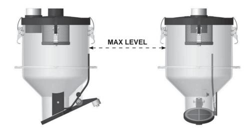
Now system is operational; an additional potentiometer adjustment may be necessary if you change, even a little bit, the specific weight or type of the fuel which has to be transported. In these cases, it is sufficient to readjust the operating time of the control panel so that it is appropriate to fill the transparent fuel dispenser tank, at each cycle, to the level indicated by the "MAX LEVEL" adhesive (see figure above).
