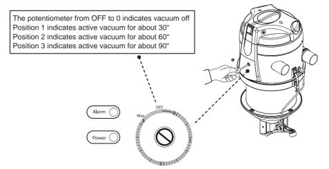
Now the vacuum unit is operational: an additional potentiometer adjustment may be necessary if you change, even a little bit, the specific weight or type of the fuel which has to be transported. In these cases, it is sufficient to readjust the operating time of the vacuum unit so that it is appropriate to fill the transparent fuel dispenser, at each cycle, to the level indicated by the "MAX LEVEL" adhesive.
