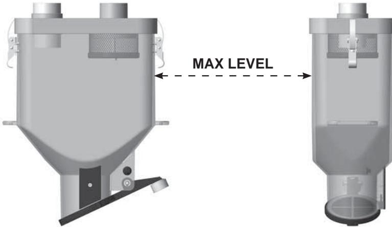
Now system is operational; an additional potentiometer adjustment may be necessary if you change, even a little bit, the specific weight or type of the fuel which has to be transported. In these cases, it is sufficient to readjust the operating time of the control panel so that it is appropriate to fill the fuel dispenser, at each cycle, to the level indicated in figure.
