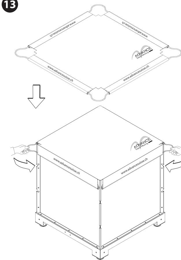
Montaggio magazzini/ Stock tanks assembly
